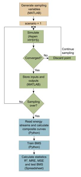
**Figure 5.** Outline of the procedure to obtain closed-form mathematical expressions: from data sampling, through simulation and data processing, to the application of the BMS and model validation.
