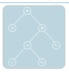
**Figure 4.** Example of a symbolic tree representing the function  $f(x) = a + (c - x_2) x_1$ .
