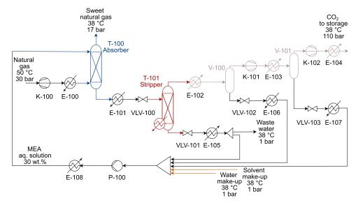
Figure 2. Natural gas sweetening process flow diagram. The process consists of an absorption stage (blue), desorption (red), CO<sub>2</sub> compression (sand), and recycle with solvent makeup (orange).
