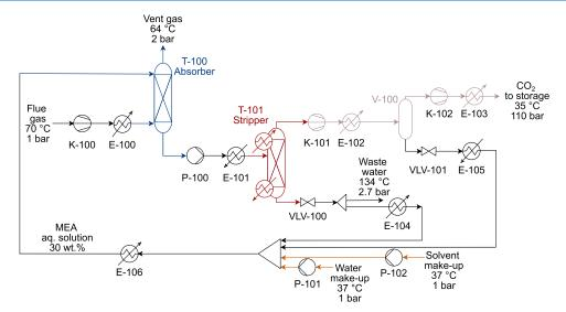
Figure 3. Flue gas treatment process flow diagram. The process consists of an absorption stage (blue), desorption (red), CO<sub>2</sub> compression (sand), and recycle with solvent makeup (yellow).
